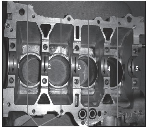
Vertical cuts for slicing of an engine block
