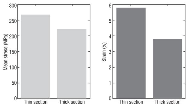
**Figure 7: Comparison of mechanical properties for thick and thin sections**
